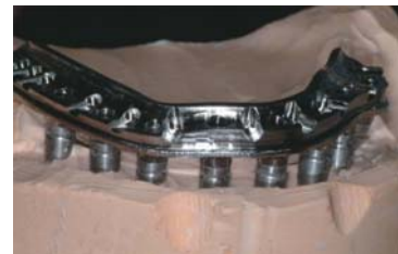
6. The design is transferred to the milling machine and the bar is milled from a solid block of titanium alloy. The CAM StructSURE™ Bar is milled with a raised lingual for retention of the denture teeth and acrylic resin. The finished CAM StructSURE Fixed-Hybrid is returned to the laboratory.
